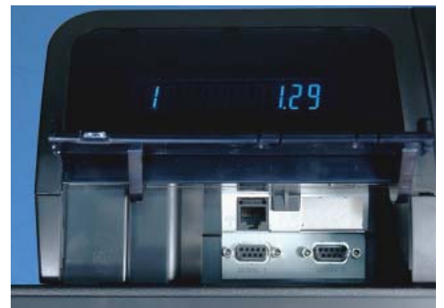
Up to Three RS-232C Ports Hidden Behind a Convenient, Easy to Access Door
