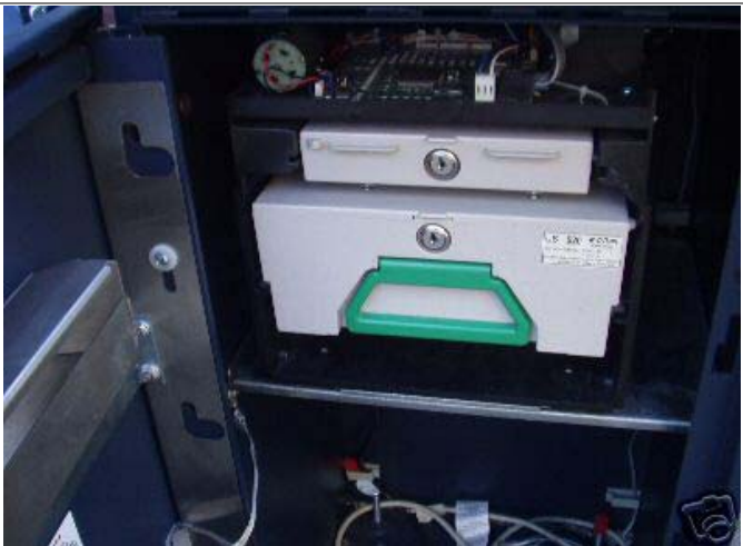
Triton 9100 cash cassette with the green handle. The reject cassette is above the cassette.
